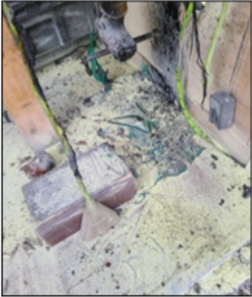
PICTURE #2 - Damage to job trailer after a battery-operated drill accidentally engaged and overheated.
